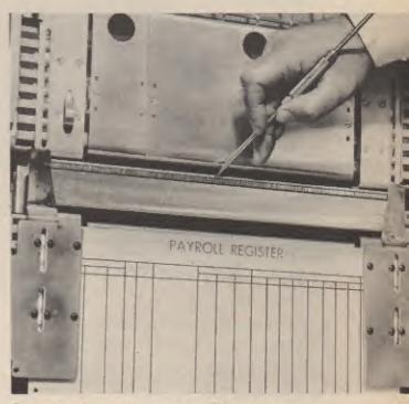
Computers for payroll register: This horizontal row of 132 electronically timed hammers taps paperforms against an inked ribbon and a fast-moving endless chain of type in an output printer of a data processing system. It prints numbers and letters at a basic speed of 600 lines a minute and, if it is operated to print numbers alone, can do it at a rate of 1,285 lines a minute.
